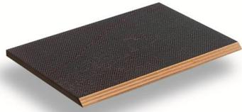
Plywood panel constructed exclusively with steamed Beech wood and surfaces covered by fire retardant resin. The coat esin increases the hardness performances, impermeability and durability of the surfaces. The edges protected by not hydroscopic vanish increase further the resistance of the water absorption.
